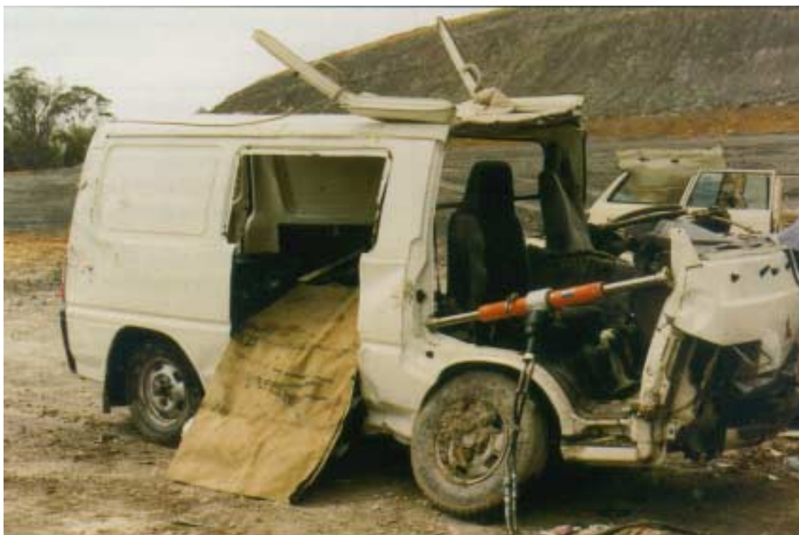
Fig 2.35 LCV Dash Roll Technique
