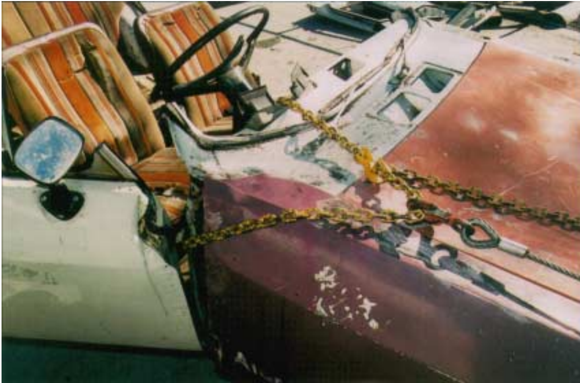
Fig 2.24 Winching the Dash Technique
