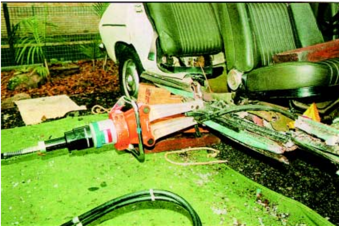
Fig 2.17 Folding Down the Sill
