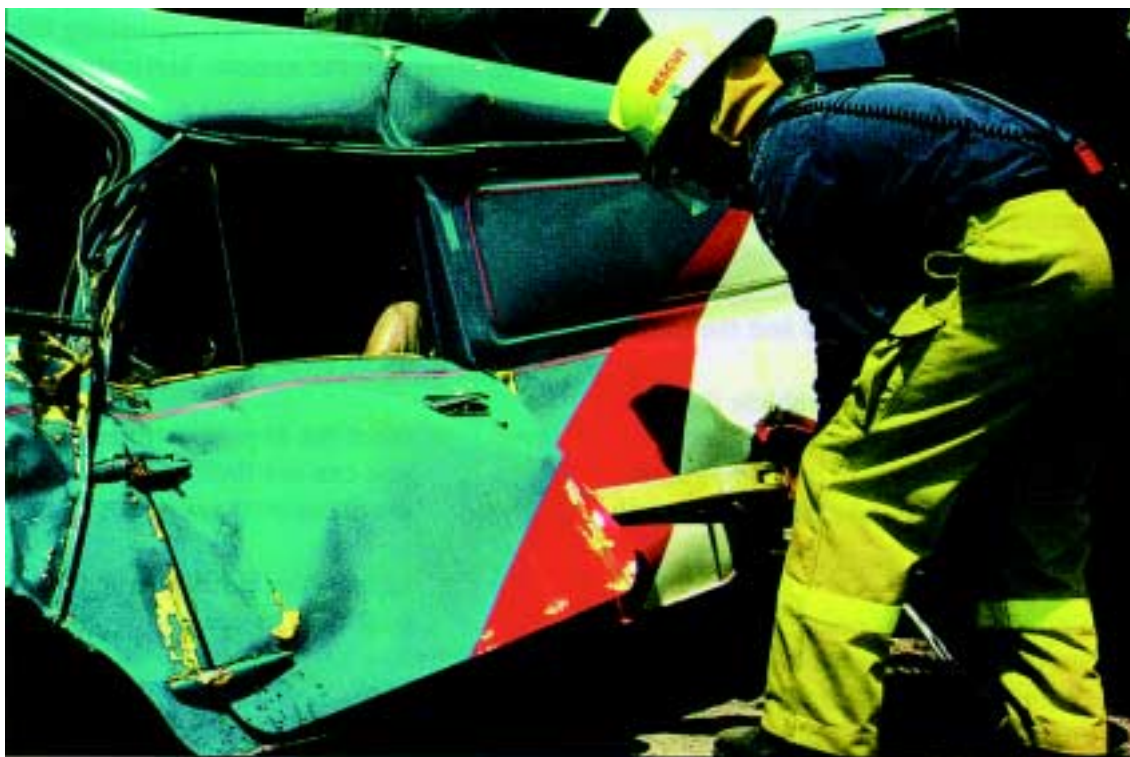
Fig 2.12 Opening Doors Using Single Action Spreaders
