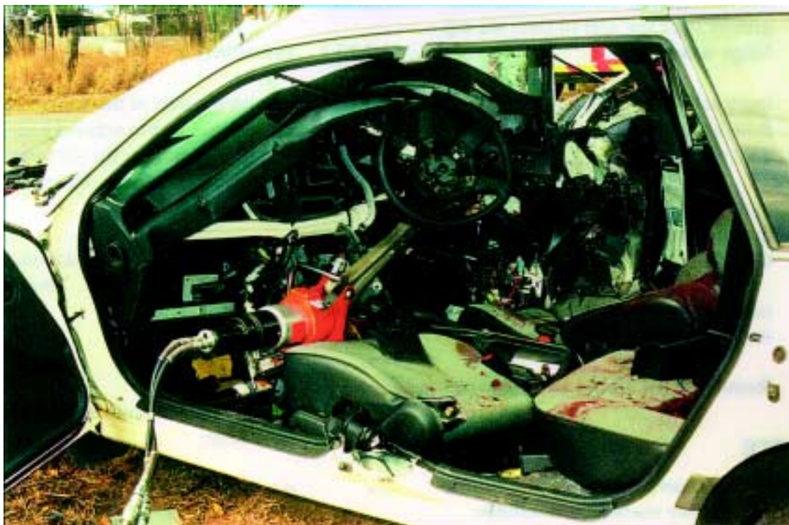
Fig 2.14 B Post Removal
