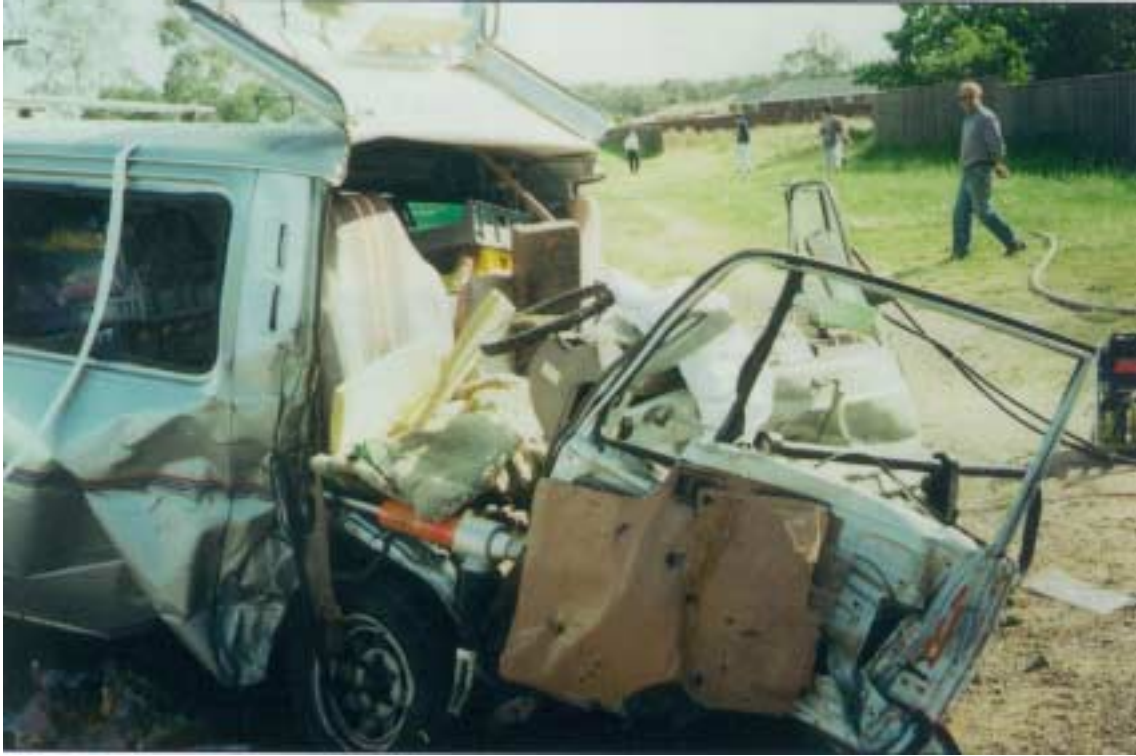
Fig 2.34 LCV Roof Flap Technique
