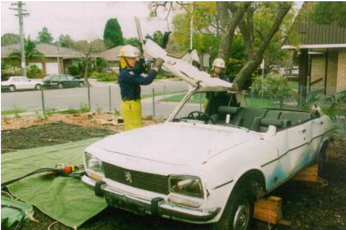
Fig 2.20 Side Roof Flapback Technique
