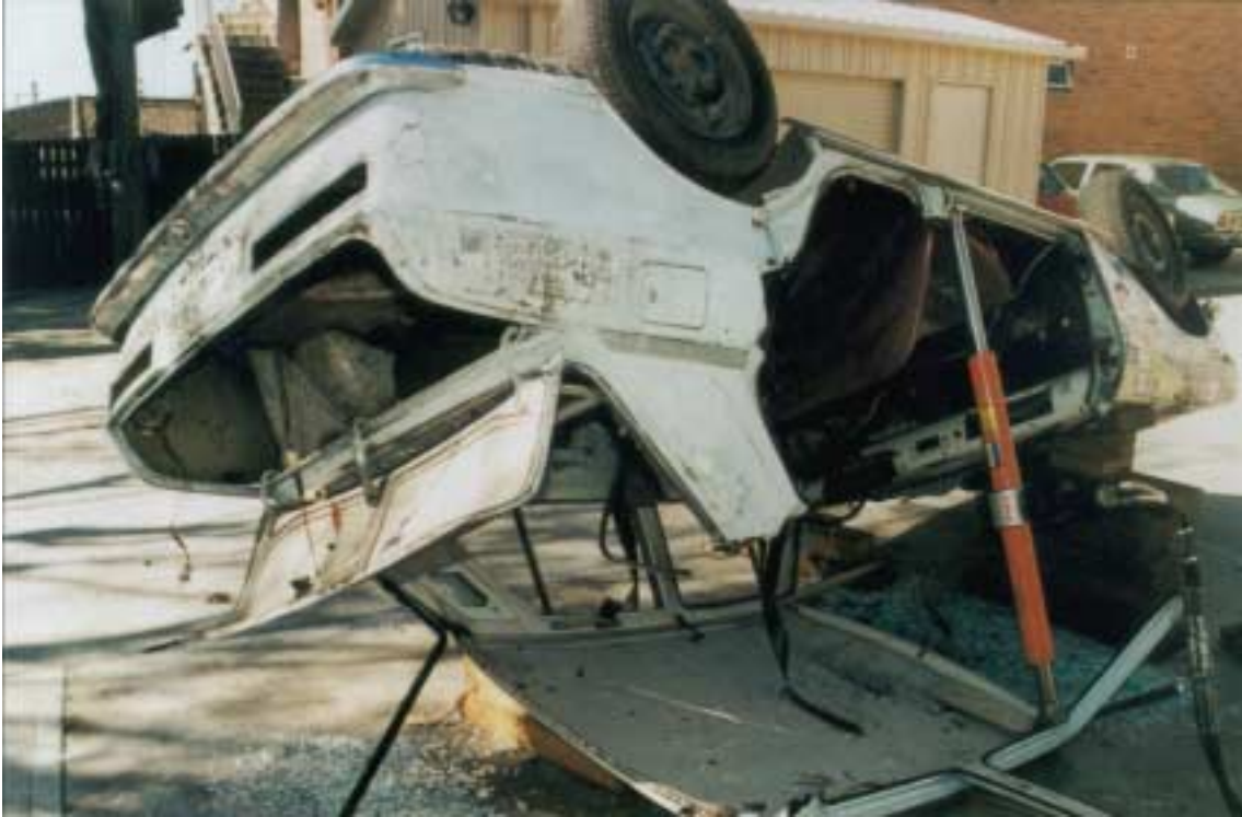
Fig 2.32 Inverted Power Ramming Technique
