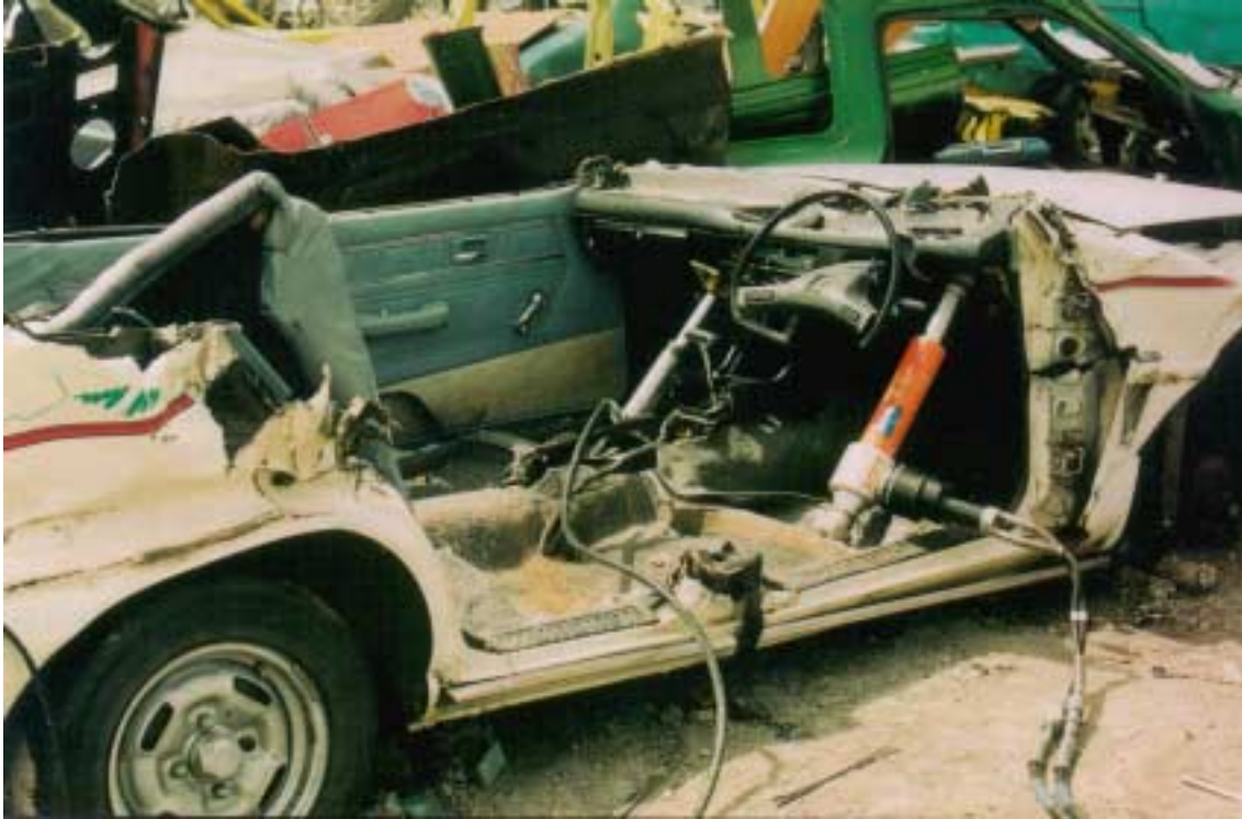
Fig 2.22 The Dash Lift Technique
