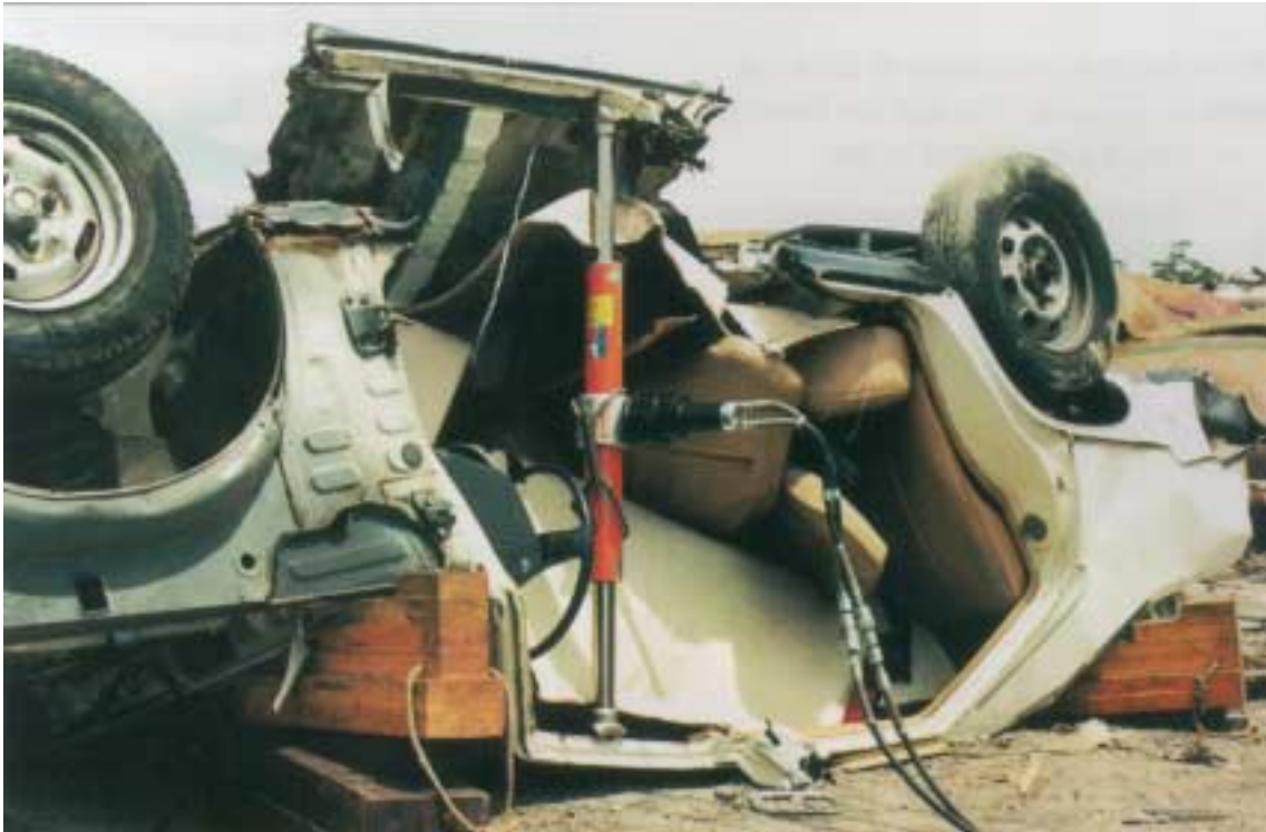
Fig 2.31 The Floorpan Flap Technique
