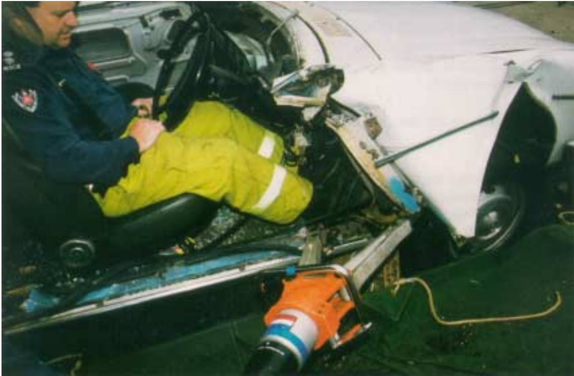
Fig 2.26 The Footwell Exposure - Method Two
