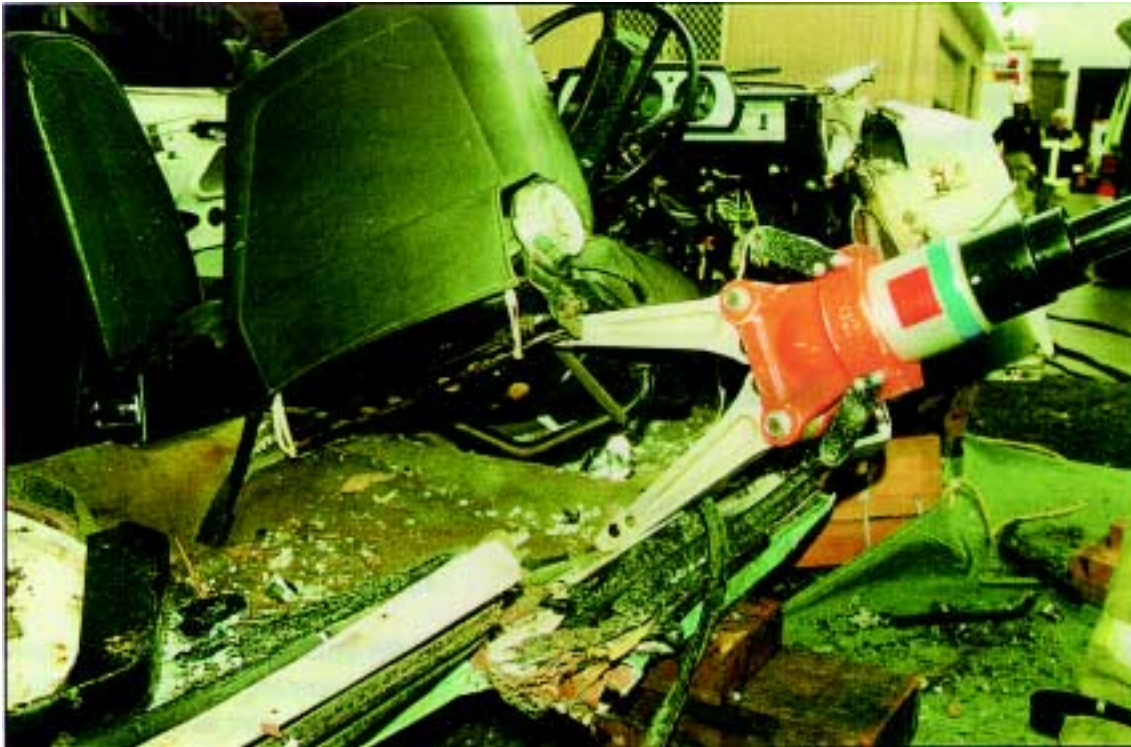
Fig 2.11 Forced Seat Removal
