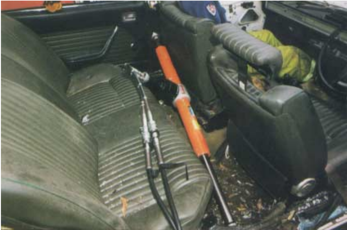
Fig 2.28 Cross Ramming Technique
