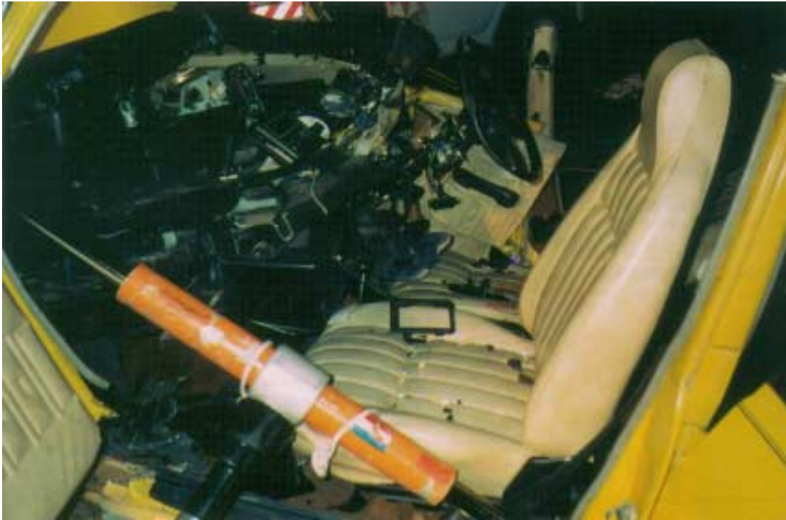
Fig 2.23 The Dash Roll Technique
