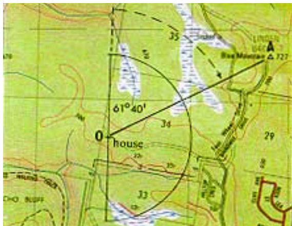
Fig 4.12 Use of the Protractor
