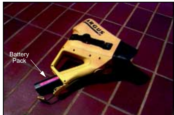
Fig 3.9 P4438 TIC and Battery Pack
