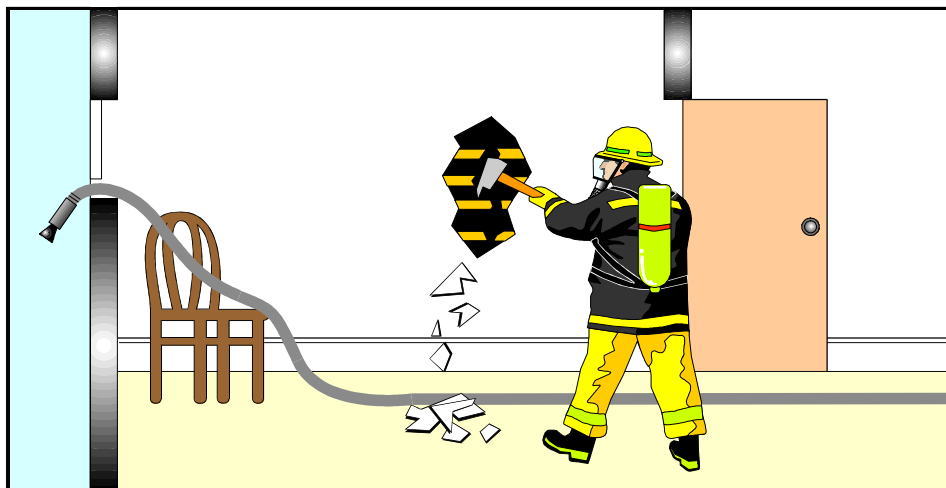
Fig 13.2 Positioning of Nozzle During Overhaul
