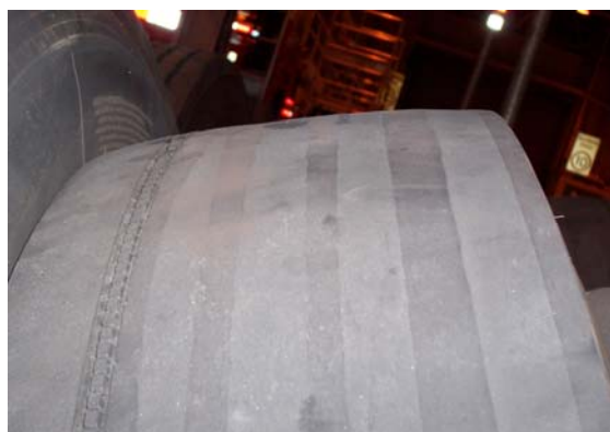
Excessively worn tyre
