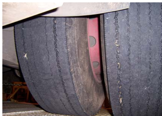
Uneven tyre wear
