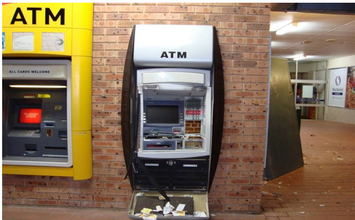
Figure 1 ATM in wall damaged by explosion
