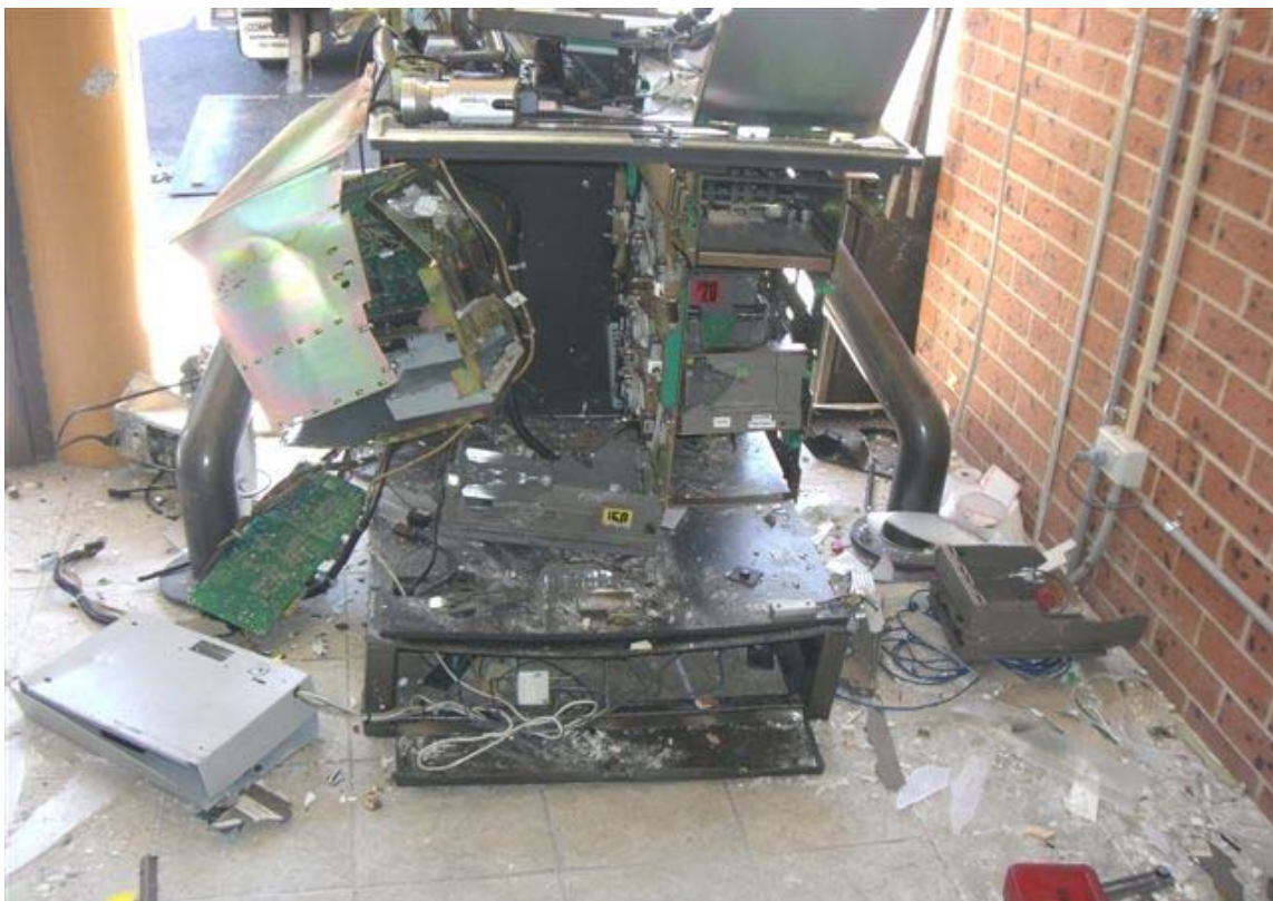
Figure 5 ATM destroyed by the explosion shown in Figure 4
