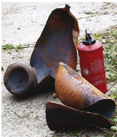
Figure 2 Ruptured acetylene cylinder found 200 m from source
